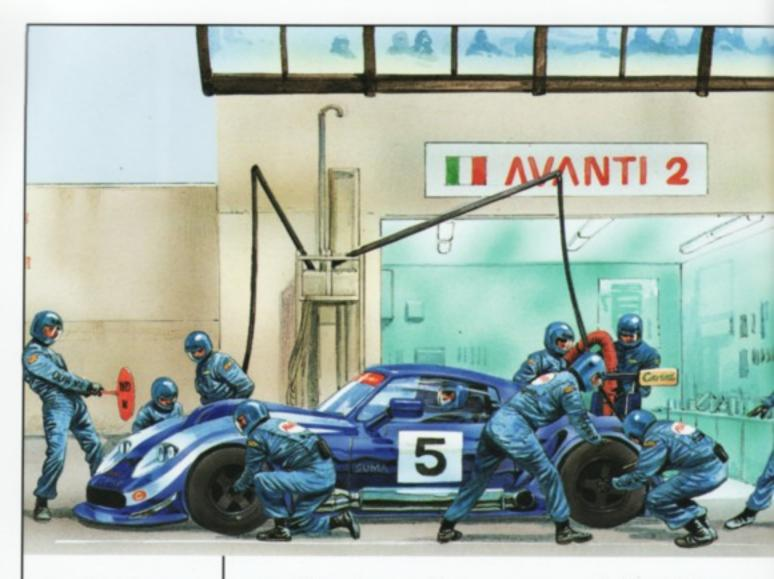
Quick change A Le Mans car can be jacked up in seconds, raising the car six inches. Each wheel is held on with just one nut. Tires are changed in the time it takes to tie a shoelace.
